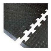
ElectraStat 180 is a static conductive material for ultimate static charge decay and ultimate static control. Type 180 features end pieces and center sections that interlock for an ESD safe floor runner of ANY length. Type 180 is provided with a diamond plate top surface over an air cell shock absorbing underside. ElectraStat 180 is designed to eliminate static generation from standing technicians and easily meets the stringent new S 20.20 standards.
