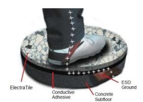
ElectraTile is a technologically advanced flooring system specifically designed to control static discharge in ESD sensitive areas. ElectraTile has conductive elements interspersed throughout the
