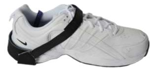
**USES:** The 109-AS ESD Heel Straps are created to provide a continuous electrical ground path between the technician and a properly grounded ESD Floor or Floor mat. Without the use of ESD heel straps a static charge can NOT make it around the insulative footwear, allowing the static charge to build on the technician and dissipate into ESD sensitive product.
