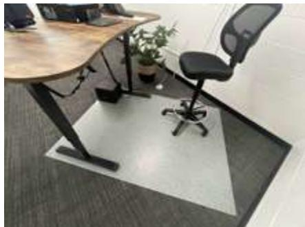
**Product Overview:** EDT-2 ESD chair mats may be manufactured to ANY rectangular or square size. They are made from a 3 mm thick interlocking modular tile that features a full surface static conductive backing covered with a topical wear surface that is nearly indestructible. We manufacture the structure at our Colorado facility by laying out your design and trimming off the interlocking outside teeth.
